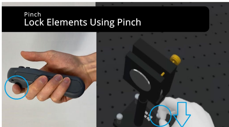
Figure 8. Lock down optical elements by pushing down a gray screw on the base plate with the trigger button.
